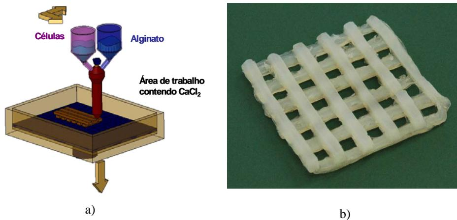
Figure 1 – Alginate-based rapid prototyping system (a), alginate scaffold structure (b).
