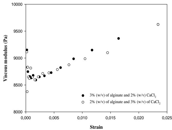
Figure 6 – Viscous modulus versus strain for two different alginate gels.
