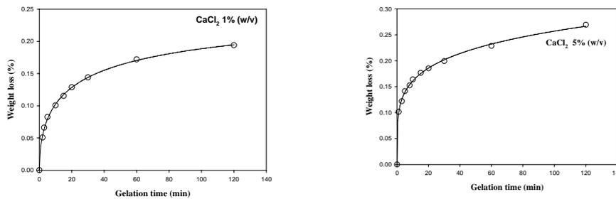
Figure 4 - Weight loss versus gelation time for a solution containing 2% (w/v) of alginate mixed with solution containing different concentrations CaCl<sub>2</sub>.
