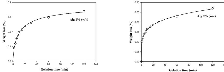
Figure 3 - Weight loss vs gelation time for two solutions containing different concentrations of alginate mixed with a solution of 5% (w/v) of CaCl<sub>2</sub>.
